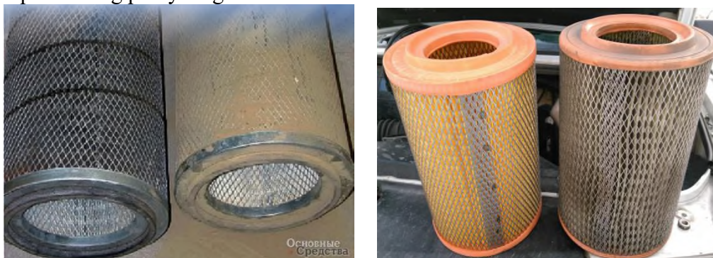
6 – rasm. BelAZ misolida karyer mashinalarining havo so‘rish tizimidagi filtrlarning ifloslanishi.
