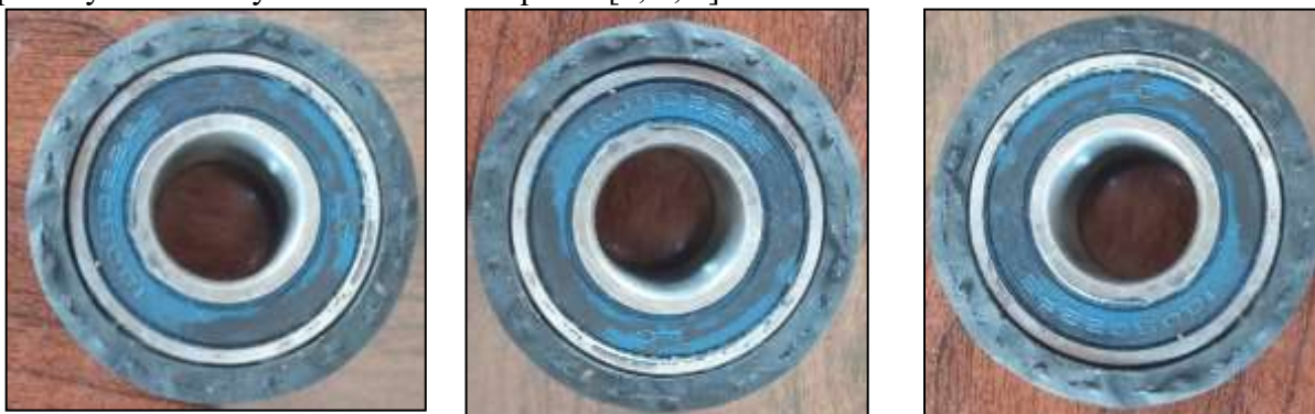
a - 7B-54MBC markali rezinadan tayyorlangan vtulka, b - 7IRP13-46 markali rezinadan tayyorlangan vtulka, c - 7IRP13-48 markali rezinadan tayyorlangan vtulka 1 - rasm. Har xil markali rezinadan tayyorlangan podshipnik vtulkasi.
